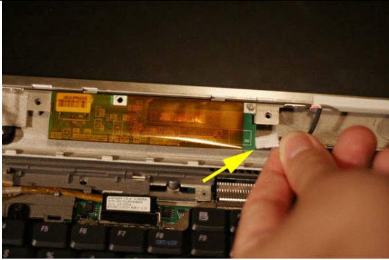
Pull out this guy, don't pull from the cable!
